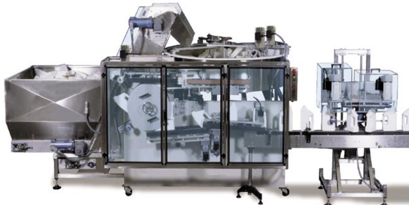
NEHHBT-72 Unscrambler with integrated secondary orienter and optional hopper elevator
